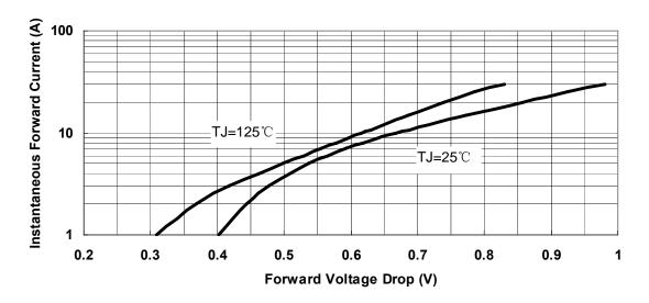
Fig.3-Typical Instantaneous Forward Voltage Characteristics
