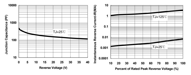
**Fig.1-Typical Junction Capacitance**
