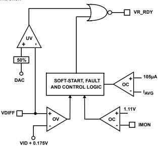
FIGURE 15. VR\_RDY AND PROTECTION CIRCUITRY
