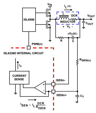
FIGURE 4. DCR SENSING CONFIGURATION
