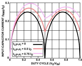
FIGURE 23. NORMALIZED INPUT-CAPACITOR RMS CURRENT vs **DUTY CYCLE FOR 2-PHASE CONVERTER**
