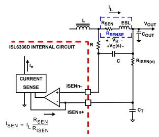
FIGURE 5. SENSE RESISTOR IN SERIES WITH INDUCTORS
