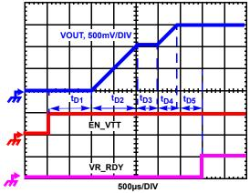
**FIGURE 14. SOFT-START WAVEFORMS**
