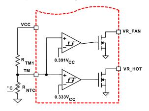
FIGURE 17. BLOCK DIAGRAM OF THERMAL MONITORING **FUNCTION**
