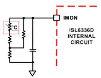
FIGURE 21. EXTERNAL TEMPERATURE COMPENSATION
