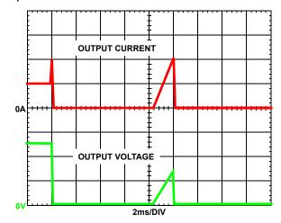
FIGURE 16. OVERCURRENT BEHAVIOR IN HICCUP MODE  $f_{SW} = 500kHz$
