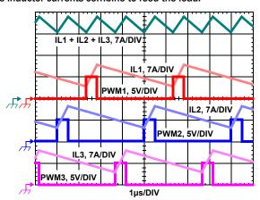
FIGURE 1. PWM AND INDUCTOR-CURRENT WAVEFORMS FOR 3-PHASE CONVERTER
