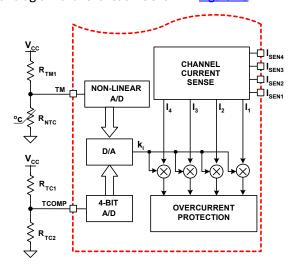
FIGURE 20. BLOCK DIAGRAM OF INTEGRATED TEMPERATURE COMPENSATION
