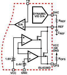
FIGURE 12. OUTPUT VOLTAGE OFFSET PROGRAMMING
