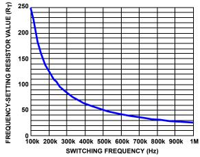
FIGURE 3. SWITCHING FREQUENCY vs RT
