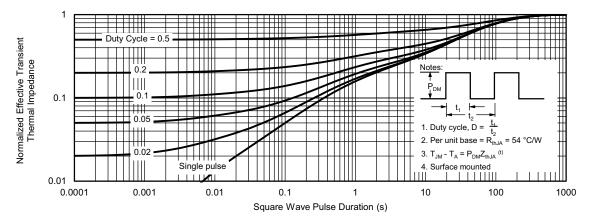
Normalized Thermal Transient Impedance, Junction-to-Ambient
