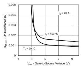
**On-Resistance vs. Gate-to-Source Voltage**
