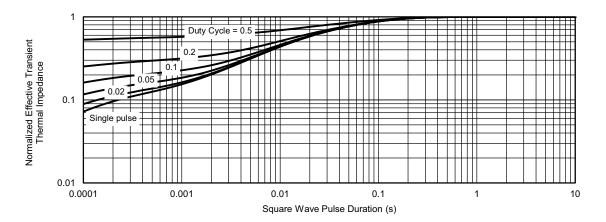
Normalized Thermal Transient Impedance, Junction-to-Case
