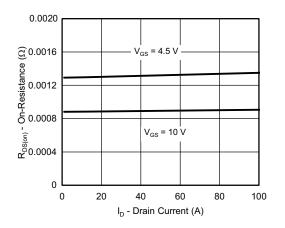
**On-Resistance vs. Drain Current**
