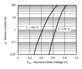
Source-Drain Diode Forward Voltage
