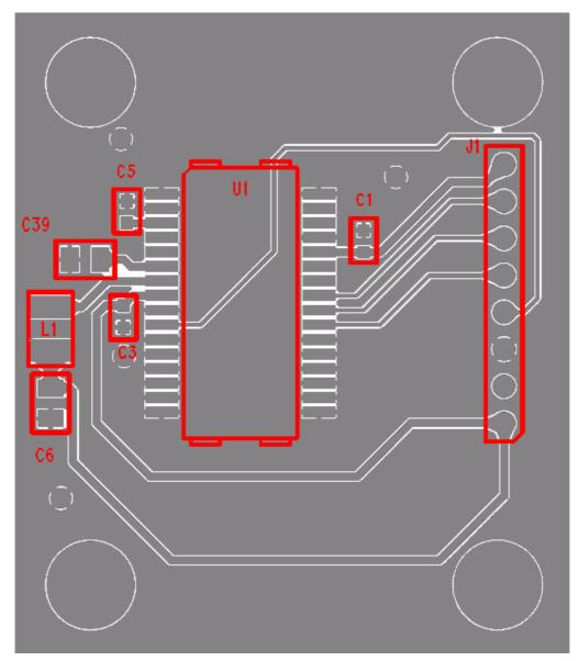
Figure 11. Example layout for SCR1100.
