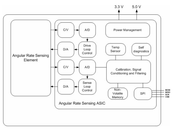
Figure 1. SCR1100 component block diagram.
