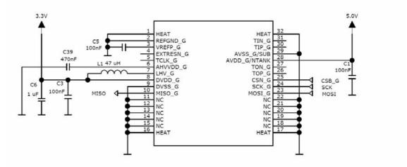
Figure 8. SCR1100 recommended circuit diagram.
