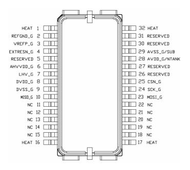
Figure 7. SCR1100 pinout diagram.
