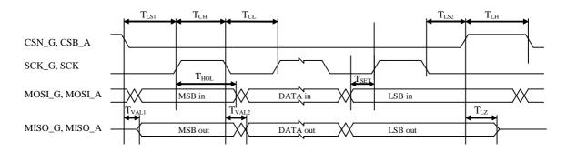
Figure 3. Timing diagram of SPI communication
