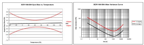
Figure 2 a) SCR1100-D04 Gyroscope offset over full temperature range, b) Allan variance curve
