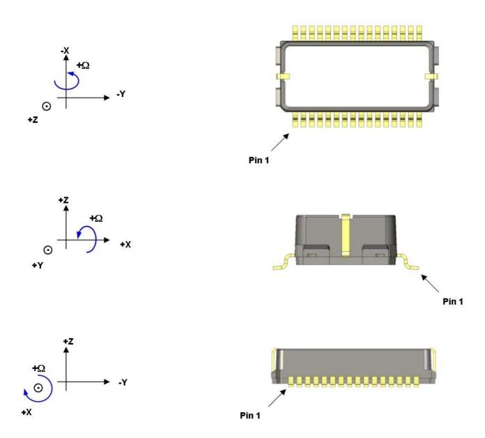
Figure 12. SCR1100 angular rate measurement direction.
