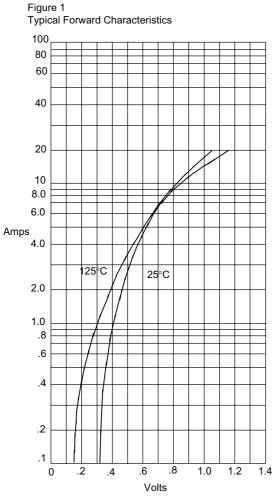
Instantaneous Forward Current - Amperesversus Instantaneous Forward Voltage - Volts
