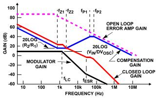
FIGURE 59. ASYMPTOTIC BODE PLOT OF CONVERTER GAIN
