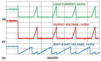
FIGURE 49. OVERCURRENT BEHAVIOR IN HICCUP MODE
