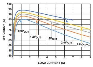
FIGURE 13. EFFICIENCY vs LOAD, VIN = 3.3V, 500kHz
