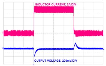
FIGURE 38. DIODE EMULATION OPERATION, V<sub>OUT</sub> = 1.2V, 125mA LOAD
