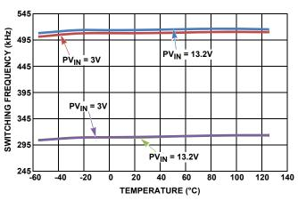
FIGURE 30. SWITCHING FREQUENCY vs TEMPERATURE
