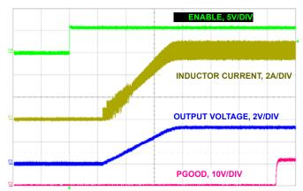
FIGURE 33. MONOTONIC SOFT-START WITH 6A LOAD, CCM
