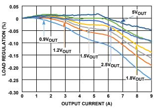
FIGURE 24. LOAD REGULATION vs V<sub>OUT</sub>, PVIN = 12V
