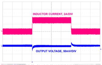
FIGURE 40. 3A LOAD TRANSIENT RESPONSE
