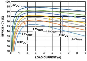
FIGURE 8. EFFICIENCY vs LOAD, VIN = 8V, 300kHz
