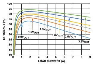
FIGURE 10. EFFICIENCY vs LOAD, VIN = 5V, 300kHz
