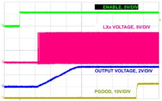
FIGURE 32. MONOTONIC SOFT-START WITH NO LOAD, CCM
