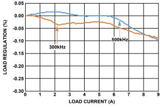
FIGURE 26. LOAD REGULATION vs SWITCHING FREQUENCY
