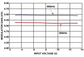
FIGURE 31. MODULATOR GAIN vs VIN
