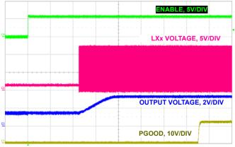
FIGURE 34. MONOTONIC SOFT-START WITH 1.5V PREBIASED LOAD
