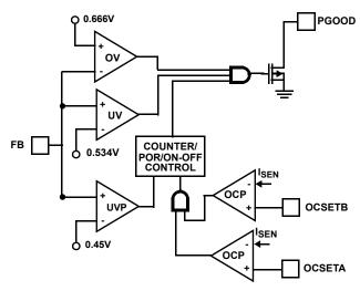
FIGURE 48. POWER-GOOD AND OC PROTECTION CIRCUITRY
