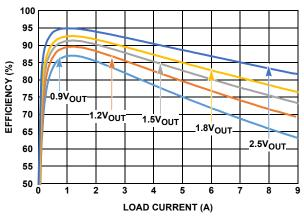
FIGURE 12. EFFICIENCY vs LOAD, VIN = 3.3V, 300kHz
