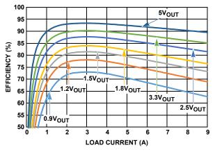
FIGURE 9. EFFICIENCY vs LOAD, VIN = 8V, 500kHz
