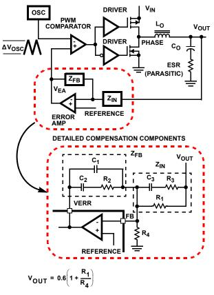
FIGURE 58. VOLTAGE-MODE BUCK CONVERTER COMPENSATION
