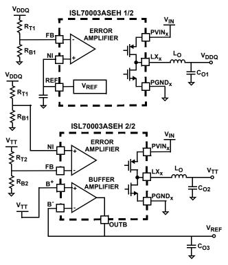
FIGURE 55. SIMPLIFIED DDR APPLICATION SCHEMATIC
