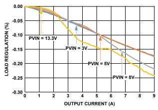
FIGURE 25. LOAD REGULATION vs PVIN, V<sub>OUT</sub> = 1.0V
