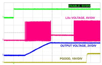
FIGURE 35. MONOTONIC SOFT-START WITH NO LOAD, DEM
