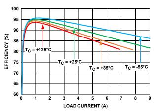
FIGURE 18. EFFICIENCY vs LOAD, VIN = 3.3V, VOUT = 2.5V, 300kHz
