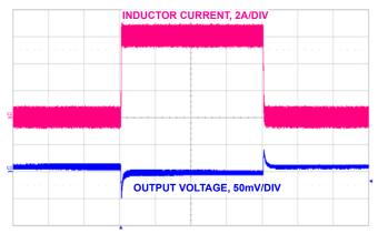
FIGURE 41. 6A LOAD TRANSIENT RESPONSE
