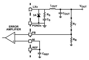
FIGURE 60. SCHOTTKY DIODE AND R-C SNUBBER
