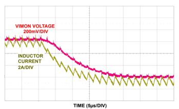
FIGURE 52. IMON RESPONSE TO 6A LOAD RELEASE
