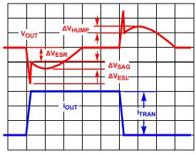
FIGURE 57. TYPICAL TRANSIENT RESPONSE
