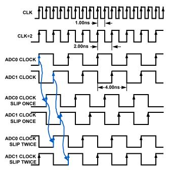
FIGURE 39. PHASE SLIP: CLK+2 MODE, f<sub>CLOCK</sub> = 1000MHz
