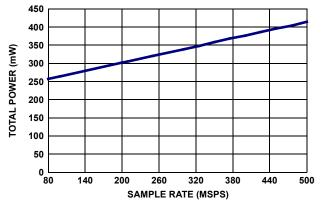
FIGURE 10. POWER vs  $f_{\mbox{SAMPLE}}$  IN 3mA LVDS MODE
