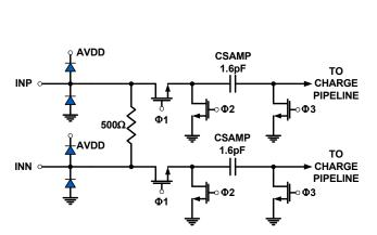
FIGURE 41. ANALOG INPUTS
