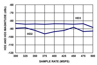
FIGURE 9. HD2 AND HD3 vs f<sub>SAMPLE</sub>
