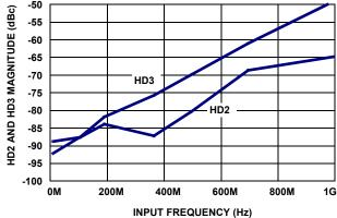
FIGURE 5. HD2 AND HD3 vs f<sub>IN</sub>
