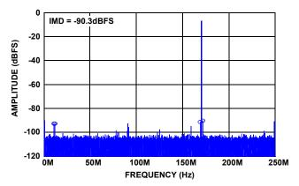
FIGURE 20. TWO-TONE SPECTRUM AT 170MHz
