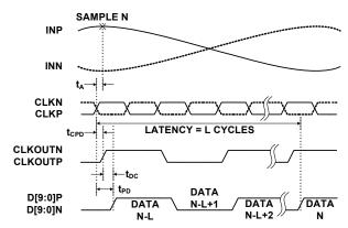
FIGURE 3. CMOS TIMING DIAGRAM (See "Digital Outputs" on page 17)
