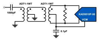
FIGURE 26. TRANSFORMER INPUT FOR GENERAL PURPOSE APPLICATIONS
