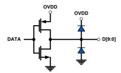
FIGURE 46. CMOS OUTPUTS
