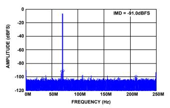
FIGURE 19. TWO-TONE SPECTRUM AT 70MHz
