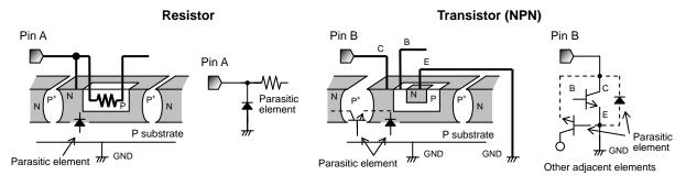
Example of monolithic IC structure
