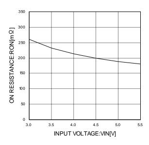
Figure 16. Switch on resistance
