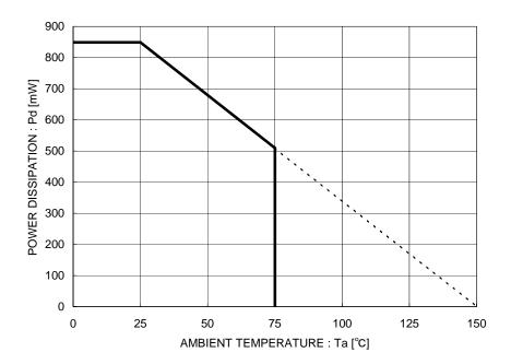
Figure 29. Power dissipation curve (Pd-Ta Curve) (HVSOF6 package)
