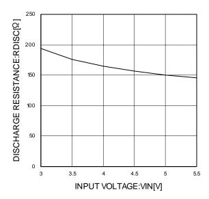
Figure 19. Discharge resistance
