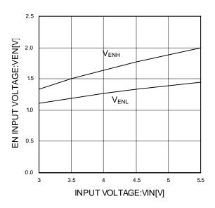
Figure 15. EN threshold voltage
