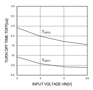
Figure 18. Switch fall time
