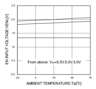
Figure 6. EN threshold voltage (Low level input voltage)
