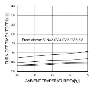
Figure 10. Switch fall time
