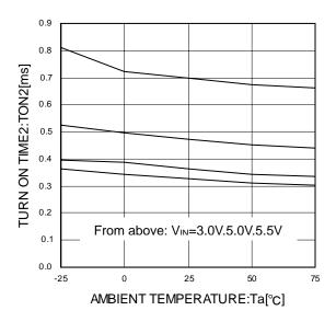
Figure 9. Switch rise delay time
