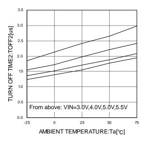
Figure 11. Switch fall delay time
