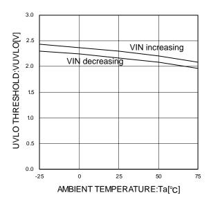
Figure 12. UVLO threshold voltage
