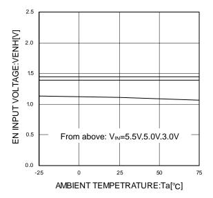
Figure 5. EN threshold voltage (High level input voltage)
