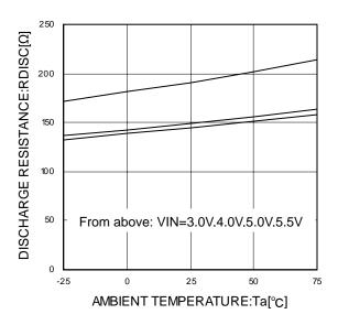
Figure 13. Discharge resistance
