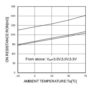
Figure 7. Switch on resistance
